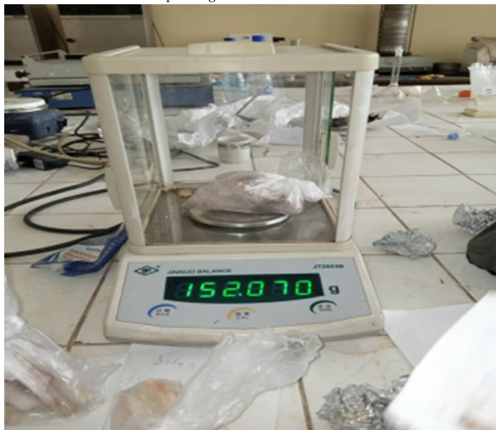
Photo 5: Measurement of kaolin sample weights
